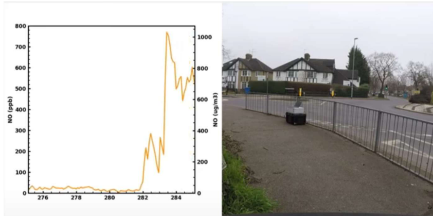
Figure 1643: NO concentration seconds after a lorry passes by the meter
